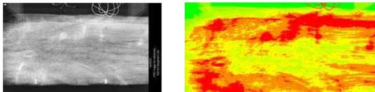
Figure 14: Sample PT23-SE2- evaluation of the object volume damage.
