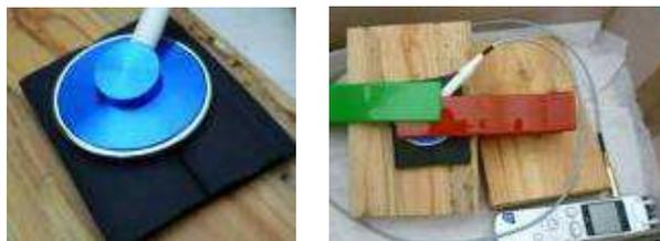
Figure 6: Measuring configuration of a fonendoscopic device for long-time recording.
