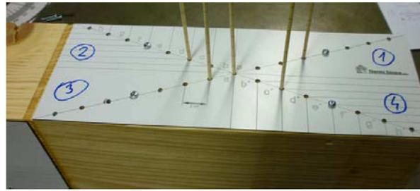
Figure 11: The measured study “A” for the localization of an object inside a biological structure (deployment of the objects is as follows:  $d_1 = 7$  cm,  $a = 6$  cm,  $c_2 = 2$  cm,  $b_3 = 12$  cm,  $c_4 = 4$  cm).
