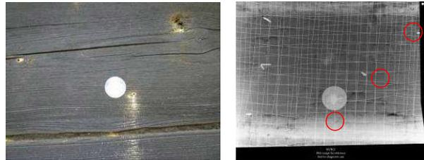
Figure 5: A sample wooden element attacked by the insect. The sample is combined with a plaster coating and netting wire; the larvae were found at spots marked by the red circles. Measured on 1 June 2012 at the gristmill in Kozlovice, the Czech Republic.
