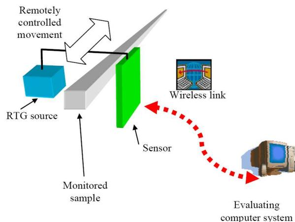
Figure 1: Diagram of the system for the monitoring of structural elements.
