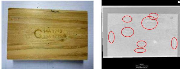
Figure 4: A sample wooden element attacked by the insect: Infested regions are marked in red.
